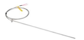
ProSense temperature sensor, Pt100 RTD, flange mount probe, 18in insertion length, 1/4in probe diameter, stainless steel sheath, mounting flange process connection, 6ft 24 AWG wire leads.
