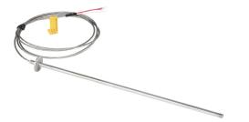
ProSense temperature sensor, Pt100 RTD, flange mount probe, 12in insertion length, 1/4in probe diameter, stainless steel sheath, mounting flange process connection, 6ft 24 AWG wire leads.
