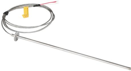
ProSense temperature sensor, Pt100 RTD, flange mount probe, 12in insertion length, 1/4in probe diameter, stainless steel sheath, mounting flange process connection, 6ft 24 AWG wire leads.
