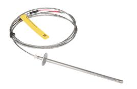
ProSense temperature sensor, Pt100 RTD, flange mount probe, 6in insertion length, 1/4in probe diameter, stainless steel sheath, mounting flange process connection, 6ft 24 AWG wire leads.
