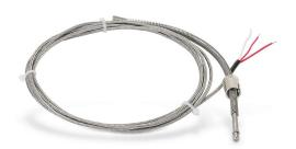
ProSense temperature sensor, Pt100 RTD, spring adjustable immersion probe, 1/4in insertion length, 3/16in probe diameter, stainless steel sheath, bayonet cap process connection, 10ft 24 AWG wire leads.
