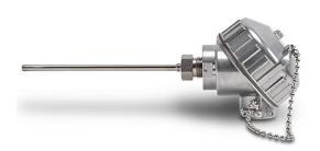
ProSense temperature sensor, Pt100 RTD, connection head probe, 18in insertion length, 1/4in probe diameter, stainless steel sheath, aluminum screw cover head with terminals.
