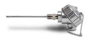
ProSense temperature sensor, Pt100 RTD, connection head probe, 18in insertion length, 1/4in probe diameter, stainless steel sheath, 1/2in male NPT process connection, aluminum screw cover head with terminals.
