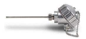
ProSense temperature sensor, Pt100 RTD, connection head probe, 12in insertion length, 1/4in probe diameter, stainless steel sheath, aluminum screw cover head with terminals.
