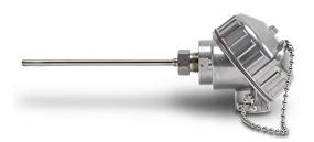
ProSense temperature sensor, Pt100 RTD, connection head probe, 6in insertion length, 1/4in probe diameter, stainless steel sheath, aluminum screw cover head with terminals.
