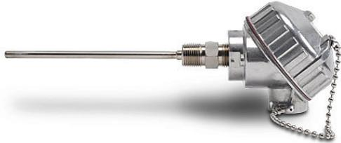
ProSense temperature sensor, Pt100 RTD, connection head probe, 6in insertion length, 1/4in probe diameter, stainless steel sheath, 1/2in male NPT process connection, aluminum screw cover head with terminals.
