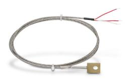
ProSense temperature sensor, Pt100 RTD, bolt-on ring, brass sheath, #12, 1/4 - 5/16in (5-8mm) screw or bolt size process connection, 6ft 24 AWG wire leads.
