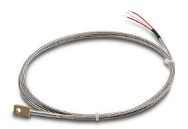
ProSense temperature sensor, Pt100 RTD, bolt-on ring, brass sheath, #6 - #10 (4-5mm) screw or bolt size process connection, 6ft 24 AWG wire leads.
