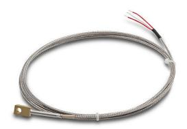
ProSense temperature sensor, Pt100 RTD, bolt-on ring, brass sheath, #6-#10 (4mm-5mm) screw or bolt size process connection, 6ft 24 AWG wire leads.
