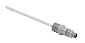
ProSense temperature sensor, Pt100 RTD, M12 probe, 150mm insertion length, 6mm probe diameter, stainless steel sheath, 1/2in male NPT process connection, 4-pin M12 quick-disconnect.
