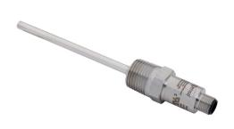
ProSense temperature sensor, Pt100 RTD, M12 probe, 100mm insertion length, 6mm probe diameter, stainless steel sheath, 1/2in male NPT process connection, 4-pin M12 quick-disconnect.
