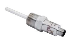
ProSense temperature sensor, Pt100 RTD, M12 probe, 50mm insertion length, 6mm probe diameter, stainless steel sheath, 1/2in male NPT process connection, 4-pin M12 quick-disconnect.
