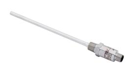
ProSense temperature sensor, Pt100 RTD, M12 probe, 150mm insertion length, 6mm probe diameter, stainless steel sheath, 1/4in male NPT process connection, 4-pin M12 quick-disconnect.
