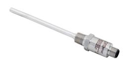
ProSense temperature sensor, Pt100 RTD, M12 probe, 100mm insertion length, 6mm probe diameter, stainless steel sheath, 1/4in male NPT process connection, 4-pin M12 quick-disconnect.
