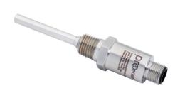
ProSense temperature sensor, Pt100 RTD, M12 probe, 50mm insertion length, 6mm probe diameter, stainless steel sheath, 1/4in male NPT process connection, 4-pin M12 quick-disconnect.
