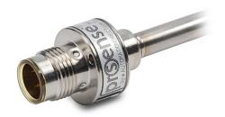
ProSense temperature sensor, Pt100 RTD, M12 probe, 160mm insertion length, 10mm probe diameter, stainless steel sheath, 4-pin M12 quick-disconnect.
