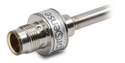
ProSense temperature sensor, Pt100 RTD, M12 probe, 360mm insertion length, 6mm probe diameter, stainless steel sheath, 4-pin M12 quick-disconnect.
