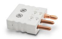
ProSense 3-pin RTD connector, standard round pin plug, 400 deg. F (200 deg. C), glass filled thermoplastic body, white, copper pins, 32 AWG to 14 AWG wire size range.
