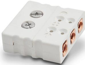
ProSense 3-pin RTD connector, standard round pin jack, 400 deg F (200 deg C), glass filled thermoplastic body, white, copper pins, 32 AWG to 14 AWG wire size range.
