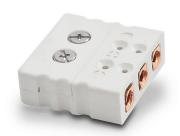
ProSense 3-pin RTD connector, standard round pin jack, 400 deg F (200 deg C), glass filled thermoplastic body, white, copper pins, 32 AWG to 14 AWG wire size range.
