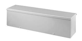
Wiegmann wiring trough, 6 x 6 x 36in (HxDxL), NEMA 1/3R, wall mount, with knockouts, carbon steel, ANSI 61 gray, powder coat finish, screw cover.
