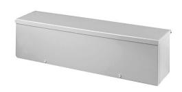
Wiegmann wiring trough, 4 x 4 x 12in (HxDxL), NEMA 1/3R, wall mount, with knockouts, carbon steel, ANSI 61 gray, powder coat finish, screw cover.
