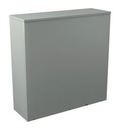
Wiegmann enclosure, NEMA 1/3R, 36 x 36 x 12in (HxWxD), wall mount, carbon steel, ANSI 61 gray, powder coat finish, screw cover, padlock hasp and staple.
