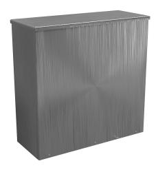
Wiegmann enclosure, NEMA 1/3R/3RX, 30 x 30 x 12in (HxWxD), wall mount, 304 stainless steel, No. 3 intermediate polished finish, screw cover, padlock hasp and staple.
