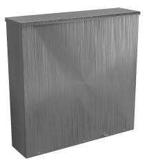
Wiegmann enclosure, NEMA 1/3R/3RX, 24 x 24 x 6in (HxWxD), wall mount, 304 stainless steel, No. 3 intermediate polished finish, screw cover, padlock hasp and staple.
