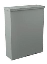
Wiegmann enclosure, NEMA 1/3R, 24 x 18 x 6in (HxWxD), wall mount, carbon steel, ANSI 61 gray, powder coat finish, screw cover, padlock hasp and staple.
