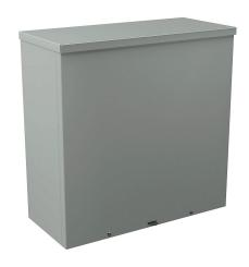
Wiegmann enclosure, NEMA 1/3R, 18 x 18 x 8in (HxWxD), wall mount, carbon steel, ANSI 61 gray, powder coat finish, screw cover, padlock hasp and staple.
