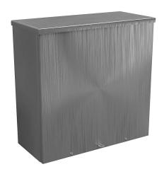
Wiegmann enclosure, NEMA 1/3R/3RX, 18 x 18 x 8in (HxWxD), wall mount, 304 stainless steel, No. 3 intermediate polished finish, screw cover, padlock hasp and staple.
