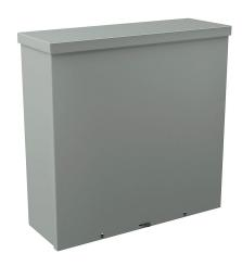
Wiegmann enclosure, NEMA 1/3R, 18 x 18 x 6in (HxWxD), wall mount, carbon steel, ANSI 61 gray, powder coat finish, screw cover, padlock hasp and staple.
