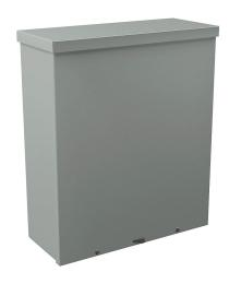
Wiegmann enclosure, NEMA 1/3R, 18 x 15 x 6in (HxWxD), wall mount, with knockouts, carbon steel, ANSI 61 gray, powder coat finish, screw cover, padlock hasp and staple.
