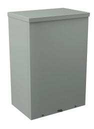
Wiegmann enclosure, NEMA 1/3R, 18 x 12 x 8in (HxWxD), wall mount, carbon steel, ANSI 61 gray, powder coat finish, screw cover, padlock hasp and staple.
