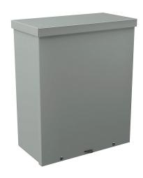
Wiegmann enclosure, NEMA 1/3R, 15 x 12 x 6in (HxWxD), wall mount, carbon steel, ANSI 61 gray, powder coat finish, screw cover, padlock hasp and staple.
