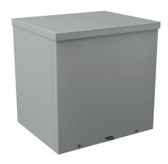
Wiegmann enclosure, NEMA 1/3R, 12 x 12 x 10in (HxWxD), wall mount, carbon steel, ANSI 61 gray, powder coat finish, screw cover, padlock hasp and staple.
