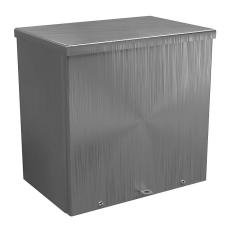
Wiegmann enclosure, NEMA 1/3R/3RX, 12 x 12 x 8in (HxWxD), wall mount, 304 stainless steel, No. 3 intermediate polished finish, screw cover, padlock hasp and staple.
