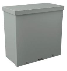
Wiegmann enclosure, NEMA 1/3R, 12 x 12 x 6in (HxWxD), wall mount, with knockouts, carbon steel, ANSI 61 gray, powder coat finish, screw cover, padlock hasp and staple.
