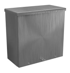
Wiegmann enclosure, NEMA 1/3R/3RX, 12 x 12 x 6in (HxWxD), wall mount, 304 stainless steel, No. 3 intermediate polished finish, screw cover, padlock hasp and staple.
