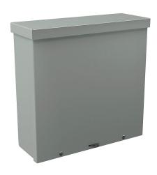
Wiegmann enclosure, NEMA 1/3R, 12 x 12 x 4in (HxWxD), wall mount, with knockouts, carbon steel, ANSI 61 gray, powder coat finish, screw cover, padlock hasp and staple.
