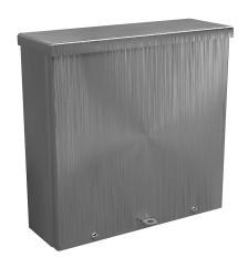
Wiegmann enclosure, NEMA 1/3R/3RX, 12 x 12 x 4in (HxWxD), wall mount, 304 stainless steel, No. 3 intermediate polished finish, screw cover, padlock hasp and staple.
