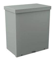
Wiegmann enclosure, NEMA 1/3R,  $12 \times 10 \times 6$  in (HxWxD), wall mount, with knockouts, carbon steel, ANSI 61 gray, powder coat finish, screw cover, padlock hasp and staple.
