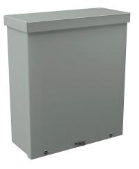
Wiegmann enclosure, NEMA 1/3R, 12 x 10 x 4in (HxWxD), wall mount, with knockouts, carbon steel, ANSI 61 gray, powder coat finish, screw cover, padlock hasp and staple.
