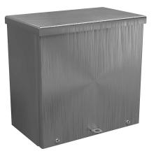
Wiegmann enclosure, NEMA 1/3R/3RX, 10 x 10 x 6in (HxWxD), wall mount, 304 stainless steel, No. 3 intermediate polished finish, screw cover, padlock hasp and staple.
