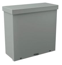
Wiegmann enclosure, NEMA 1/3R, 10 x 10 x 4in (HxWxD), wall mount, with knockouts, carbon steel, ANSI 61 gray, powder coat finish, screw cover, padlock hasp and staple.
