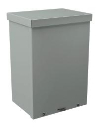
Wiegmann enclosure, NEMA 1/3R, 12 x 8 x 6in (HxWxD), wall mount, with knockouts, carbon steel, ANSI 61 gray, powder coat finish, screw cover, padlock hasp and staple.
