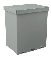
Wiegmann enclosure, NEMA 1/3R, 10 x 8 x 6in (HxWxD), wall mount, with knockouts, carbon steel, ANSI 61 gray, powder coat finish, screw cover, padlock hasp and staple.
