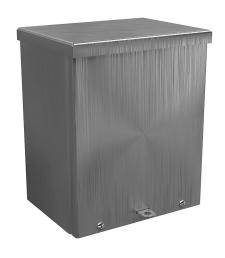
Wiegmann enclosure, NEMA 1/3R/3RX,  $10 \times 8 \times 6$  in (HxWxD), wall mount, 304 stainless steel, No. 3 intermediate polished finish, screw cover, padlock hasp and staple.
