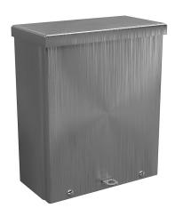
Wiegmann enclosure, NEMA 1/3R/3RX, 10 x 8 x 4in (HxWxD), wall mount, 304 stainless steel, No. 3 intermediate polished finish, screw cover, padlock hasp and staple.
