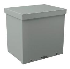
Wiegmann enclosure, NEMA 1/3R, 8 x 8 x 6in (HxWxD), wall mount, with knockouts, carbon steel, ANSI 61 gray, powder coat finish, screw cover, padlock hasp and staple.
