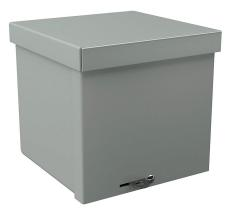
Wiegmann enclosure, NEMA 1/3R, 6 x 6 x 6 in (HxWxD), wall mount, with knockouts, carbon steel, ANSI 61 gray, powder coat finish, screw cover, padlock hasp and staple.
