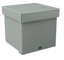
Wiegmann enclosure, NEMA 1/3R, 4 x 4 x 4 in (HxWxD), wall mount, with knockouts, carbon steel, ANSI 61 gray, powder coat finish, screw cover.
